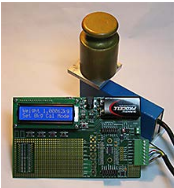
Figure 2. Weigh Scale System Setup Using the AD7190
